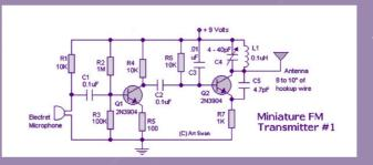
This is a small test-transmitter with a radial outreach of ca. 50m on a functional platina illustration....
